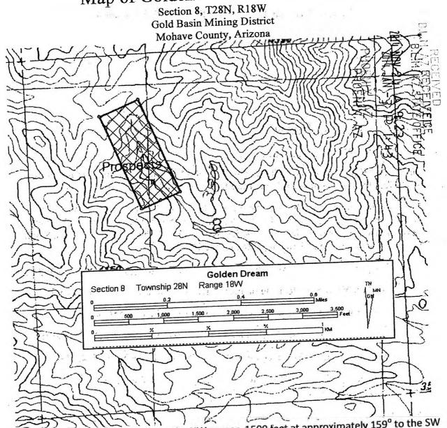
The Claim is delineated thusly: From the NW corner, 1500 feet at approximately 159° to the SW corner, then 600 feet at approximately 69° to the SE Corner, then 1500 feet at approximately 339° to the NE corner, then 600 feet at approximately 249° to the point of beginning.
